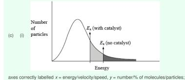
graph showing correct curve for Maxwell-Boltzmann distribution; If two curves are drawn, first and second mark can still be scored, but not third. Curve(s) must begin at origin and not go up at high energy. two activation energies shown with Ecat shown lower; Award the mark for the final point if shown on an enthalpy level diagram. (ii) catalyst provides an alternative pathway of lower energy / OWTTE; Accept catalyst lowers activation energy (of reaction).
